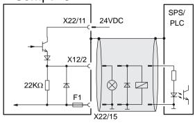
The outputs are short circuit proof; a short circuit generates an error.
